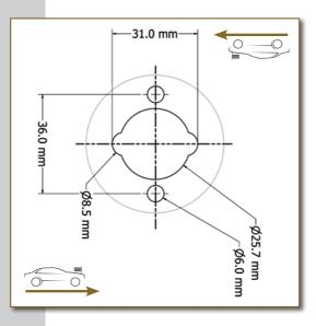
However, some modern cars use very thin sheet metal for the fender, so the fender might become deformed if you use too much force while inserting the flag pole. To avoid this, add strong supports which will decrease the risk of damaging the car. For one example, see image below. This bracket was made for a Toyota Landcruiser-Station J20-VDJ200.
