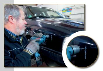
Increase the size of the middle hole to 25.7 mm. Using a step drill might help you. Enlarge the hole at the left and right side with a file so that the base and its 2 bolts will fit.
